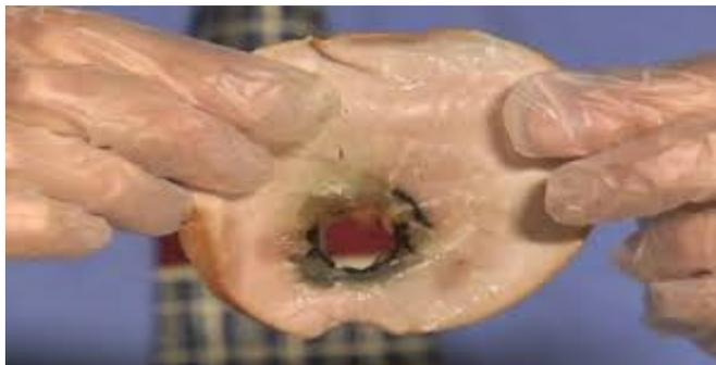
*The burning effect of a button battery when placed between slices of ordinary ham, simulating a child's throat.*
